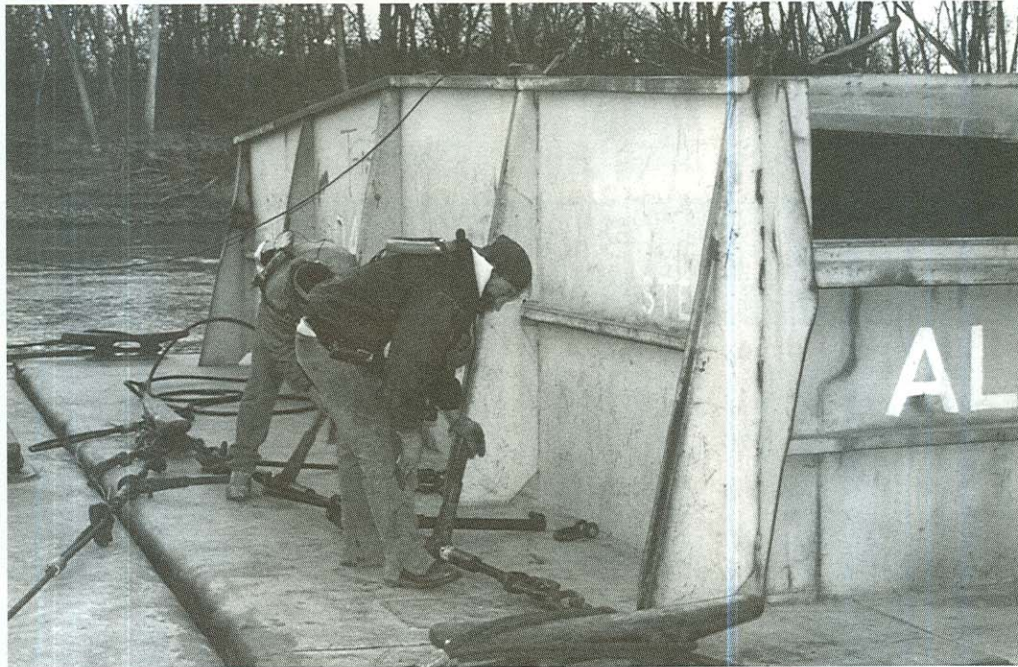
Crew members of the Missouri towboat, the Omaha , wire barges together. Photo by Mark Knudsen
