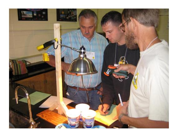
Surface Composition and Temperature (Cups of dry soil, moist soil, and water)
